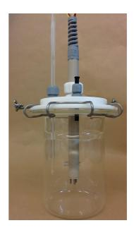
The Bubble test Cell has been designed for the everyday testing of oilfield inhibitors on steel. It is suitable for standard Bubble test work or for LCM<sup>™</sup> techniques that in addition to the average corrosion rate vs. time gives information pertaining to Localised Corrosion.
